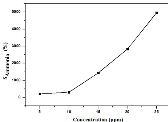
Figure 5: Sensing response variation of MgO film for different ammonia concentration
