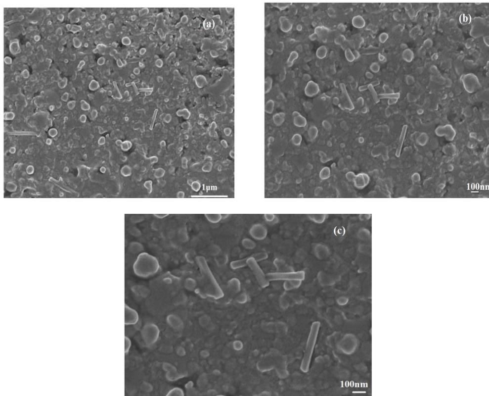
Figure 3: Field-emission scanning electron micrograph of MgO thin film at different magnification (a) 20,000 (b) 30,000 (c) 40,000
